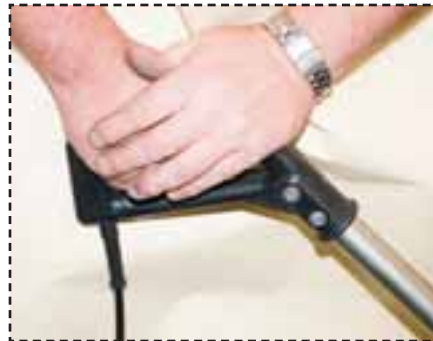
Fig.26: Improper use of handle extension.
