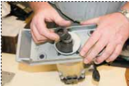
Fig.32: Remove rubber protection cup.
