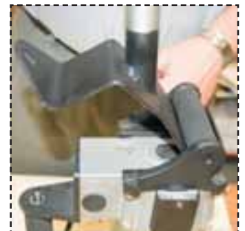
Fig.21: Make sure that extension hooks on securely to top handle.
