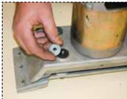
Fig.40: Replacing washers and bushing to top enclosure.
