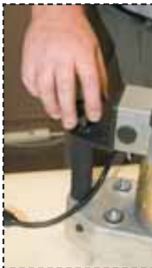
Fig.18: Removing the back handle attachment knob
