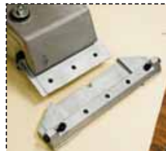
Fig.10: Fit extension assembly to vibrating plate.
