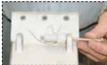
Fig.44: Remove and inspect axle bolt.
