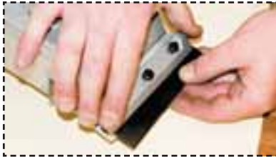
Fig.4: Inserting the blade in between the support mount and vibrating plate.
