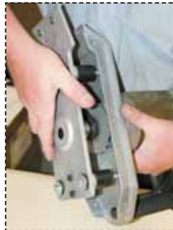
Fig.31: Removing the vibrating plate.
