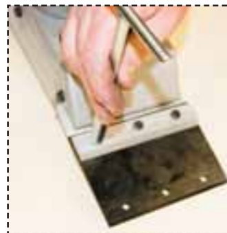
Fig.7: Tightening nuts with nut driver
