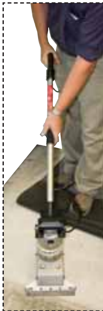
Fig.25: Proper use of the SAMURAI with handle extension.
