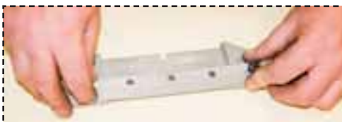
Fig.9: Fasten support mount to plate extension.
