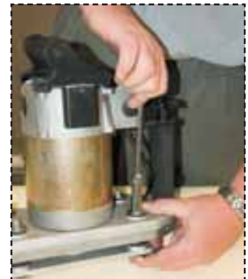
Fig.41: Tighten nut caps.
