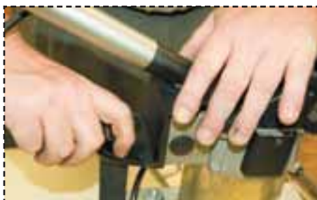
Fig.22: Re-attaching the back handle attachment knob to secure handle extension to unit.
