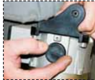
Fig.43: Carefully remove brush caps.
