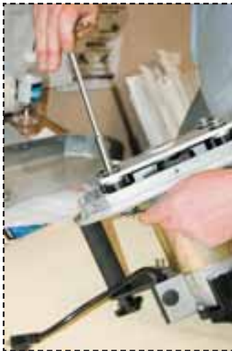
Fig.30: Safely support the SAMURAI when in inverted position.
