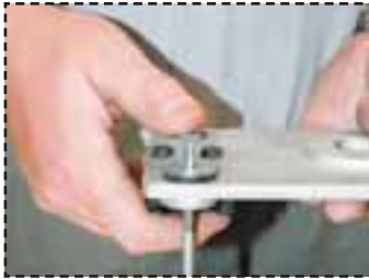
Fig.35: Insert bolts through vibrating plate.
