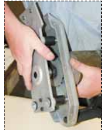
Fig.38: Align bolts on vibrating plate to holes on top enclosure.
