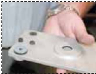
Fig.34: Replace washers and bushings
