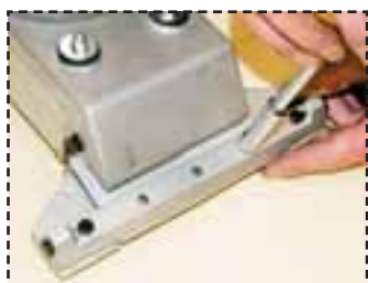
Fig.11: Bolt extension to machine.
