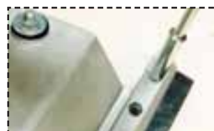
Fig.13: Tightening nuts with nut driver
