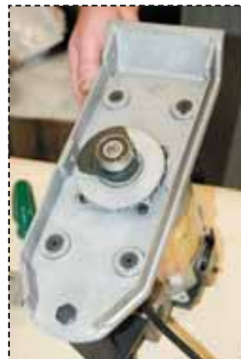
Fig.33: Location of counterweight.
