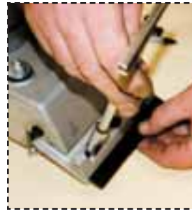
Fig.5: Tightening nuts with nut driver
