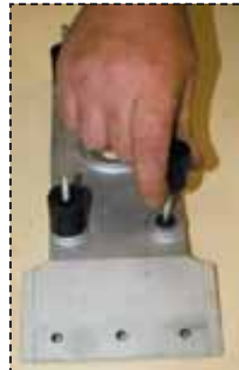
Fig.37: Slide large rubber bushings as shown.
