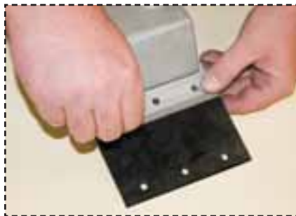
Fig.6: Align holes on support mount to blade.
