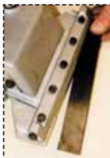
Fig.12: Slide blade in between support mount and extension plate.
