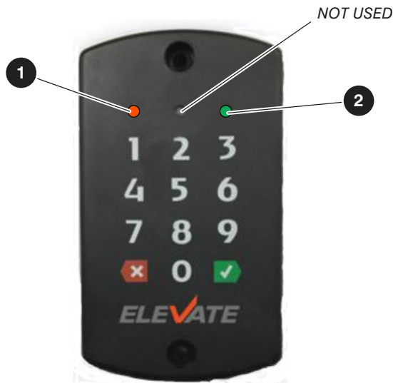
Figure 06 Keypad of the access control unit
